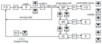
The keyboard code can be set to zero by holding the SET key and turning the controller off then on again.
